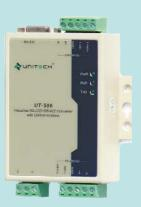
RS-485 SIGNAL REPEATER & RS-232 CONVERTER
